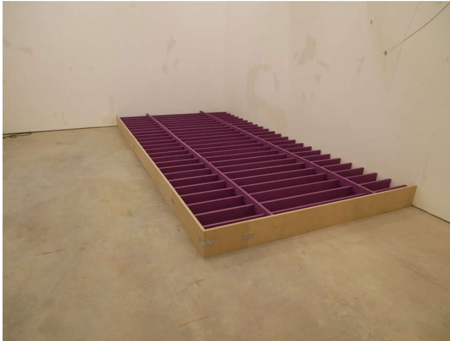
Picture 1: Photography of test specimen 1 in the reverberation room.
