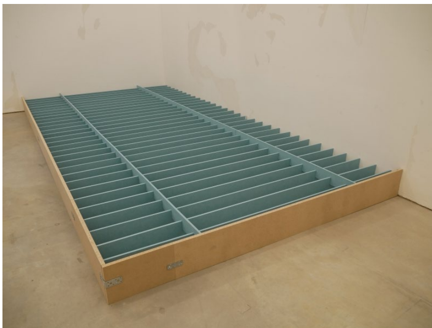
Picture 2: Photography of test specimen 2 in the reverberation room.
